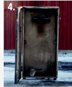
4. After 5 minutes it was safe to open the cabinet and let the non-toxic potassium aerosol out.
