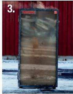
3. The active MAUS aerosol fills the space and stops the fire instantly and the temperature drops to 40°C in seconds.
